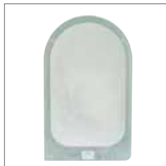
Flat glass after 1.5 years near a motorway, with DynaClean
