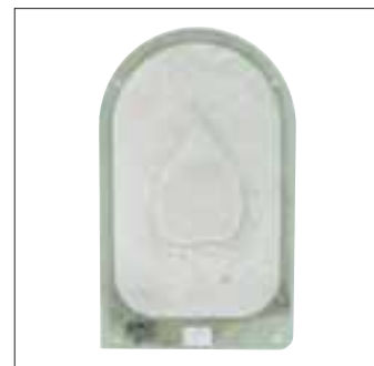
Flat glass after 1.5 years near a motorway, without DynaClean
